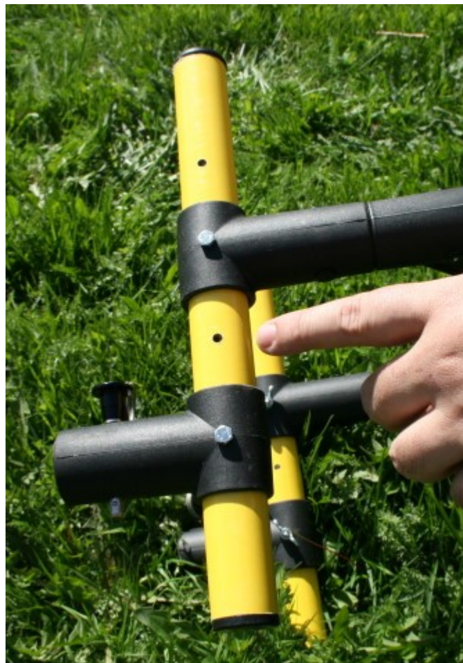
Fig. 16 Holes for the adjustment of the parallel position
