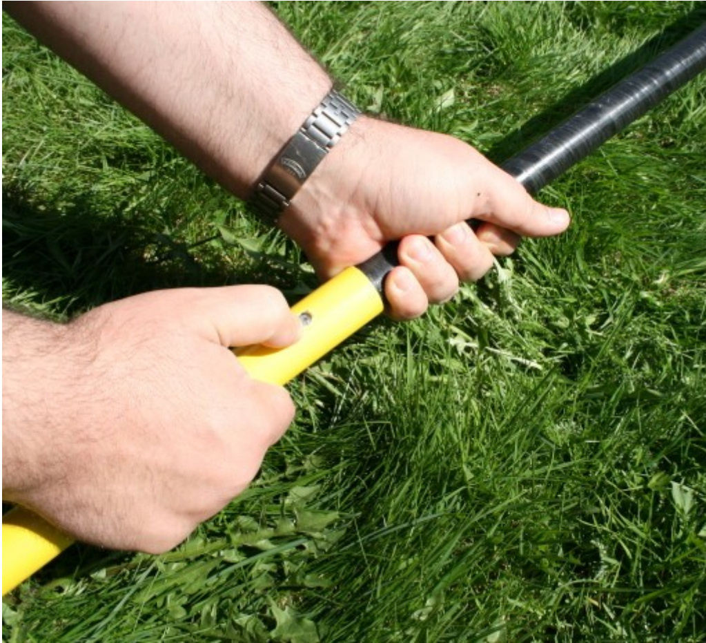
Fig. 10 Insert the antenna holder into the front antenna holder connector.
