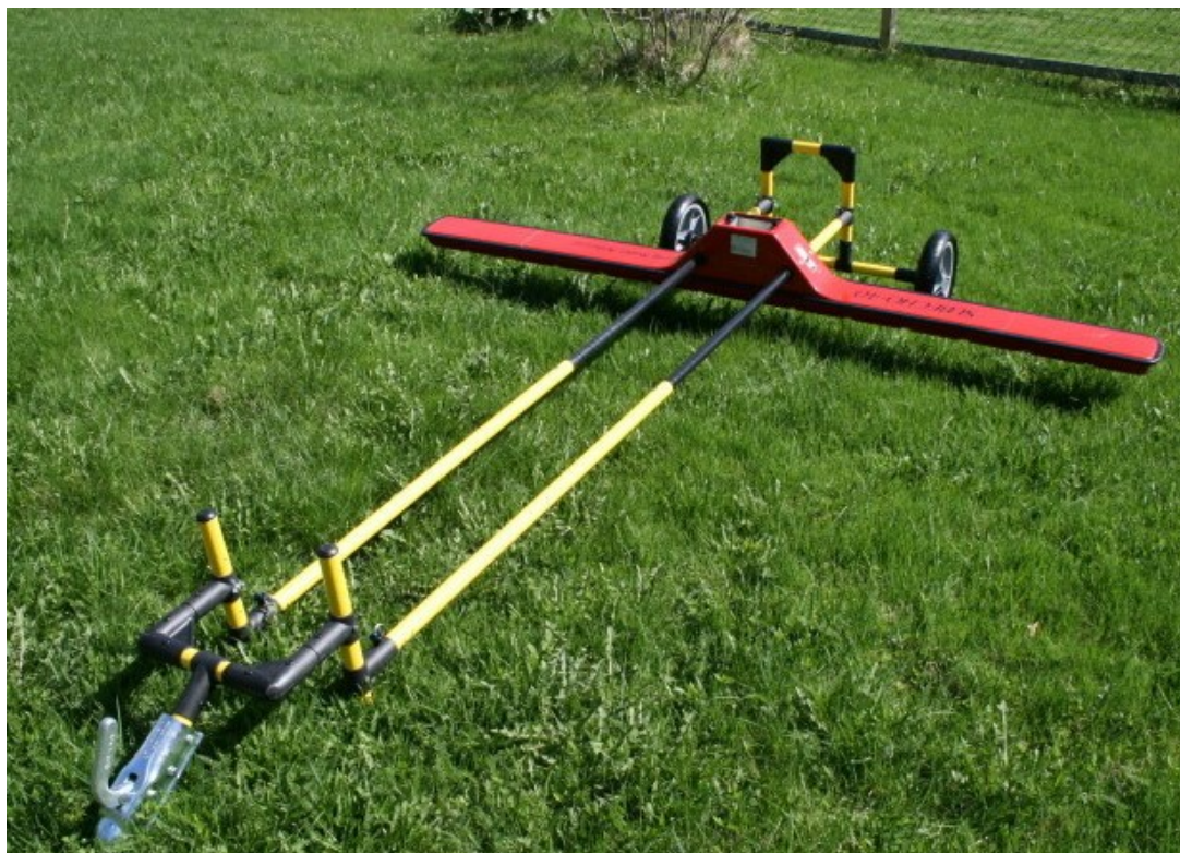
Fig. 14 GPR Trailer kit with antenna attached , front view
