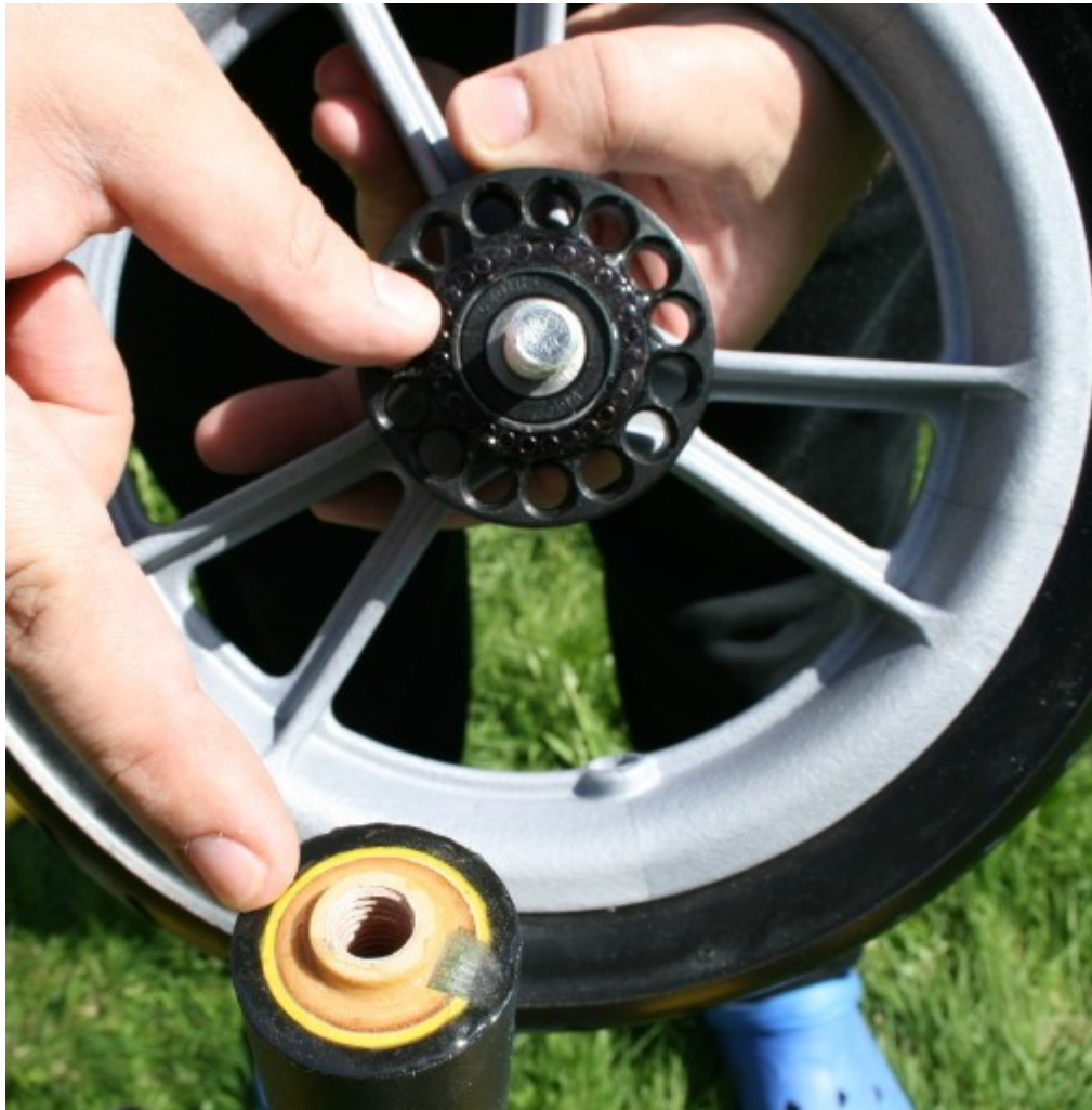
Fig. 7 Encoder wheel and encoder mounted in the rear axis.
