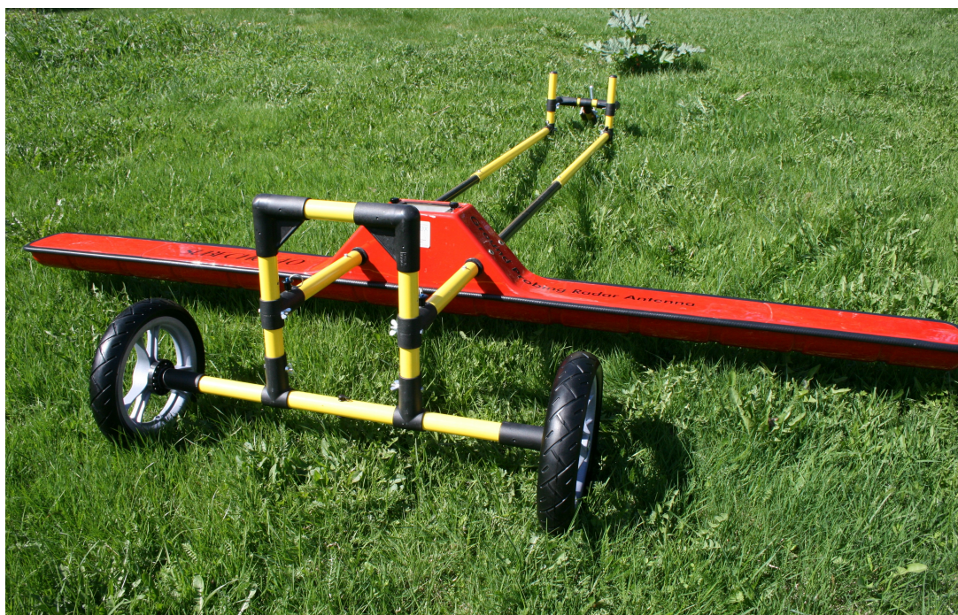
Fig. 15 GPR Trailer kit with antenna attached, rear view
