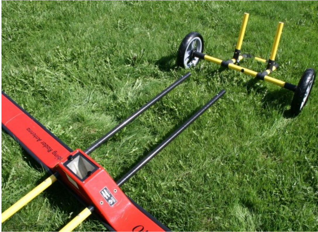
Fig. 12 Mounting the antenna in the antenna holders.
