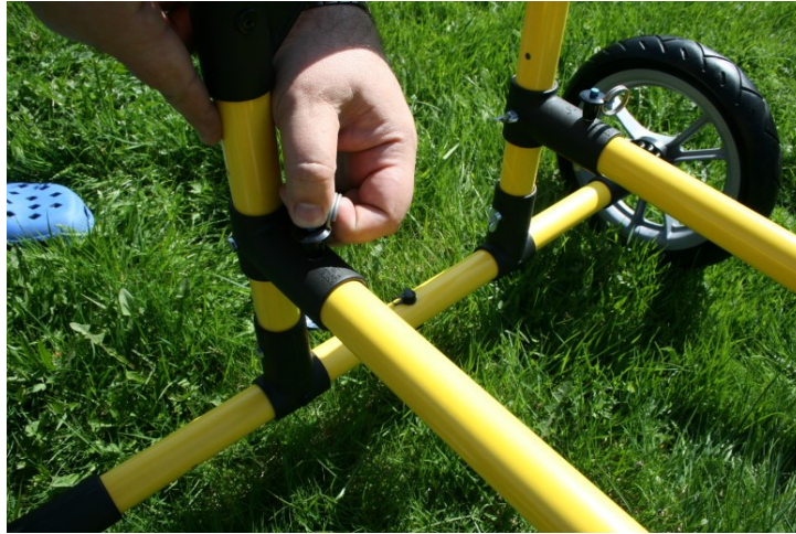
Fig. 8 Securing rear antenna holders with pins.
