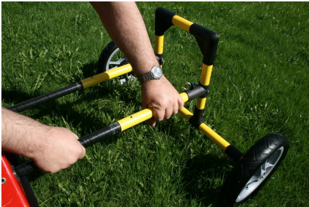
Fig. 13 Assemble the antenna holders into the rear connectors.
