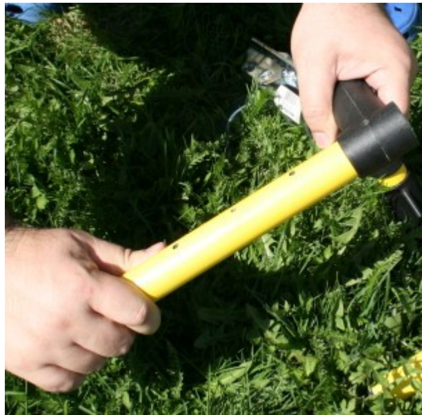
Fig. 2 Insert front bar in hitch ball assembly.
