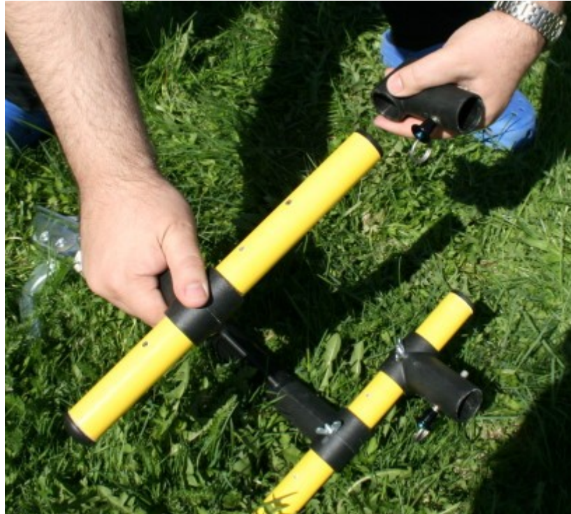
Fig. 4 Insert back the antenna holder connectors.
