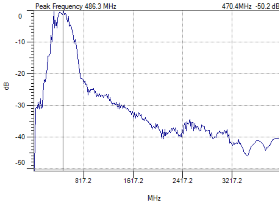
Fig.2 Power Spectrum of the GCB-500 ground coupled antenna.
