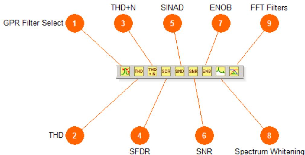
These are a set of automatic and semiautomatic measurement tools based upon the spectrum loaded in the spectrum data view.
