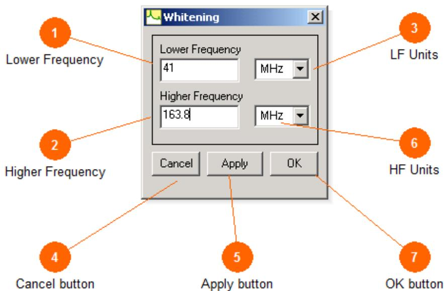
Enter in this dialogue box the values for the lower and upper frequencies of the desired pass-band to apply whitening.
