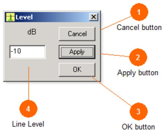
Use this dialogue box to select the level for the reference line on the spectrum data view.
