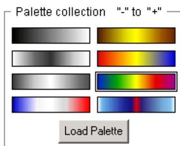
In this window the set of available palettes are displayed and is possible to select existing palettes or to load new ones. GaiaSpectrum® uses standard Windows® palettes with extension PAL. It is important though that all colors are present and no cells are skipped.
