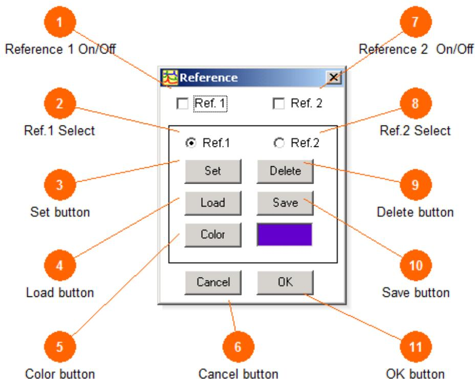
The reference setup button invokes a new window with all the options for setting reference functions. This is a useful editing tool when two or three different phase responses must be compared to each another.
