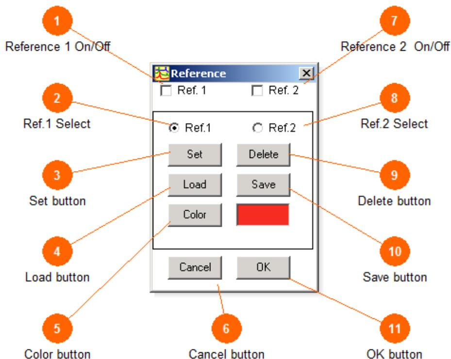
The reference setup button invokes a new window with all the options for setting reference waveforms. This is a useful editing tool when two or three different traces most be compared to each other.
