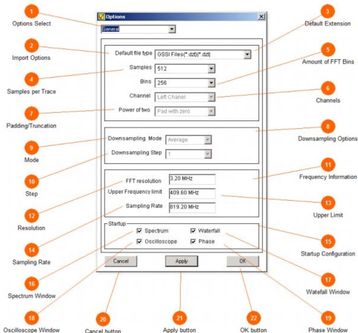
The options menu allows you to control how the imported file are processed and accessed.
