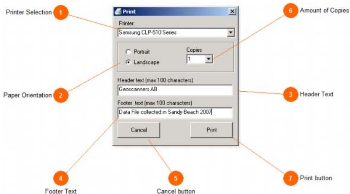
Setup the basic printing options for the active data view. When the printer dialogue box is invoked the active data view will be maximized automatically.
