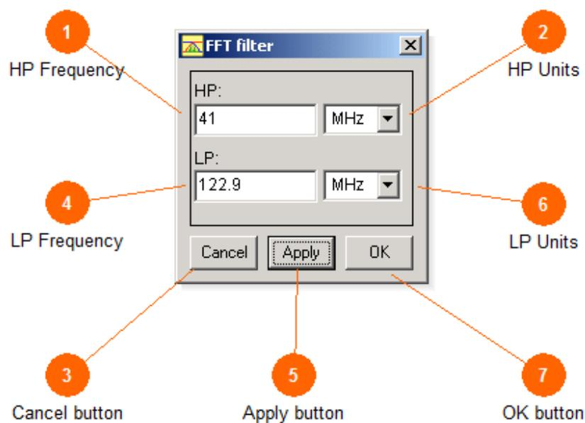
Enter in this dialogue box the low and high cut-off frequencies for the FFT filter. By combining these settings any kind of filter response can be achieved.
