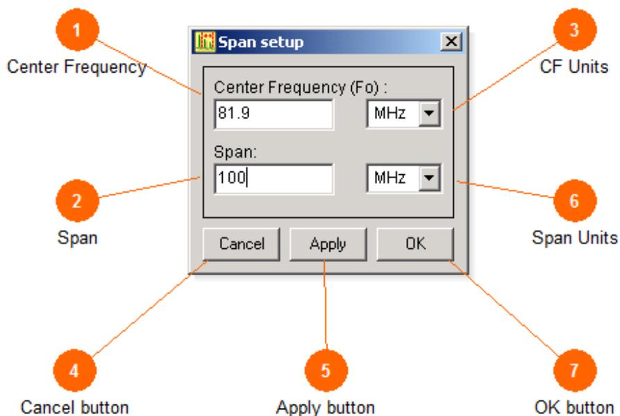
The span setup button invokes a new window that allows for selecting a portion of the spectrum function in the spectrum data view. In such a way it is easy to observe and measure a specific portion of the spectrum in a greater detail. If the span setup button is depressed then the spectrum data view shows the entire frequency span from zero to the maximum available frequency component.
