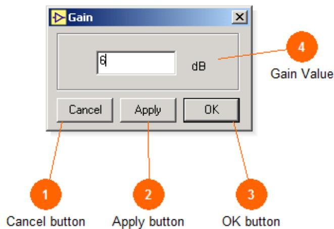
This dialogue box is used to enter the desired amount of amplification to apply to the current data set.
