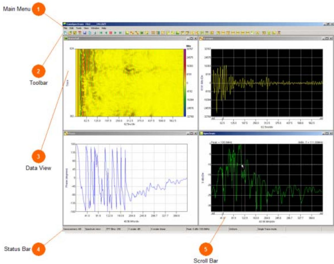
The main window of GaiaSpectrum® has the main menu, the toolbar, the data view or views and the status bar. The spectrum and o-scope data views have both a scroll bar that allows for moving the data back or forward in order to find troublesome areas.
