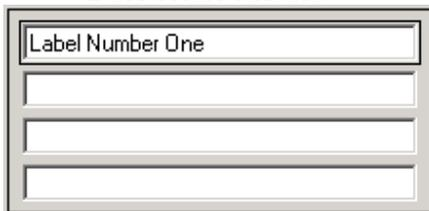
This box contains four labels that can be edited. The text box with a frame around it is selected. All the changes done with the clear, font and write buttons will affect only the label contained within the selected text box. To select a text box point at it with the mouse and press the left button.
