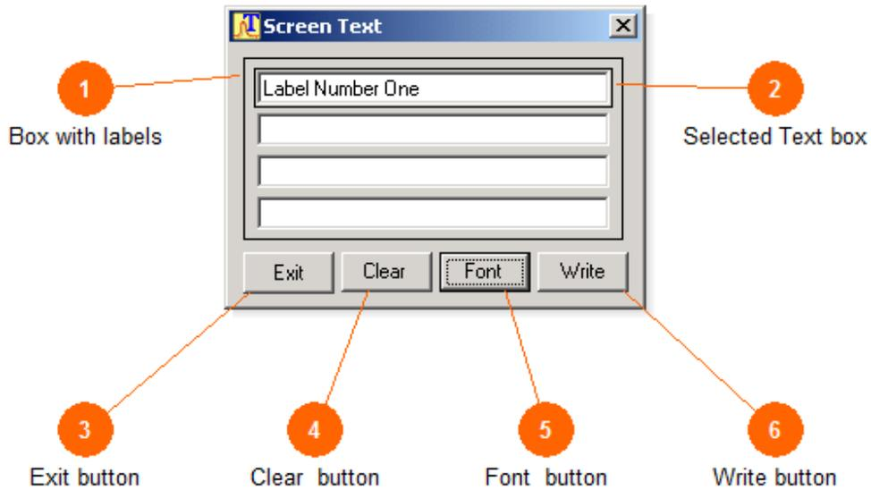
Dialogue box for entering and formatting labels to be displayed on the spectrum, o-scope, phase or waterfall data view.
