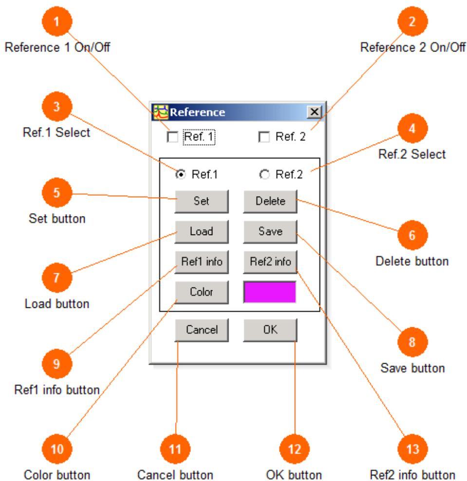
The reference setup button invokes a new window with all the options for setting reference spectrum lines. This is a useful editing tool when two or three different spectrum must be compared to each other.
