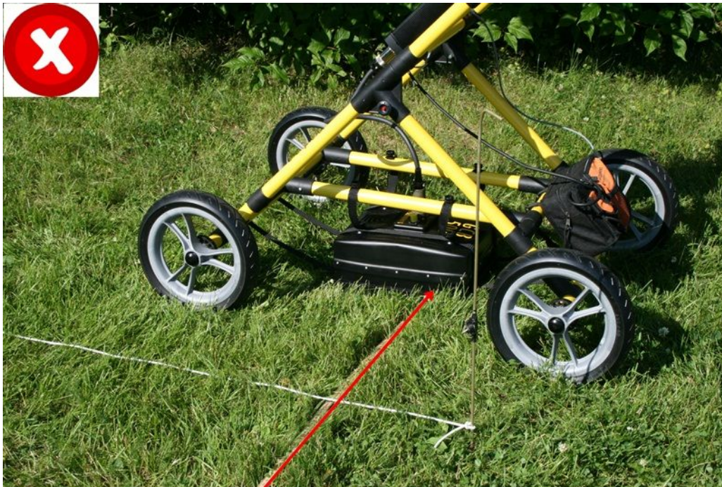
After declaring the baseline, ALL profiles of the grid must start at the same baseline!
