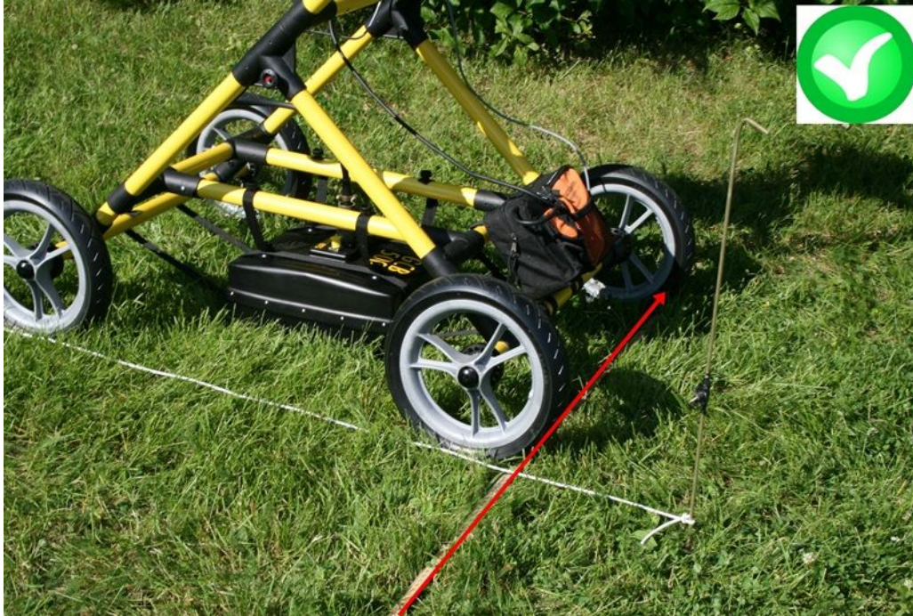
After declaring the baseline, ALL profiles of the grid must start at the same baseline!
