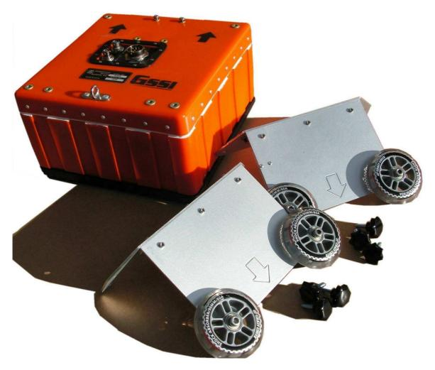
The kit contains two halves, one for each side of the antenna and a set of thumb screws for fastening them to the antenna.
